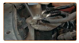
Unscrew the fasteners of the fuel filter housing cover. Use Torx T15. Use a ratchet wrench.
