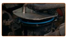
Remove the fuel filter. Use a flat screwdriver.
