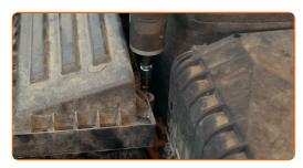
Remove the fender protection cover.
