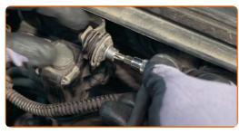
6 Unscrew the brake fluid reservoir cap.
