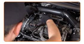
Secure the wiring of the ignition coils in its mounting seats.
