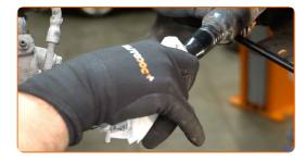
Remove the CV joint circlip. Use a flat screwdriver.
