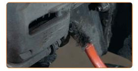
Unscrew the brake caliper fastening. Use a combination spanner #13. Use a combination spanner #15. Use a drive socket #13. Use a ratchet wrench.
