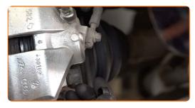
Install the brake caliper retaining spring.
