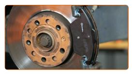
Replacement: brake pads - VW Passat B8 Variant (3G5, CB5). Tip:
