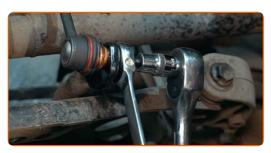
Tighten the fastener connecting the stabilizer link to the shock strut. Use a combination spanner #18. Use a drive socket #18. Use XZN #6. Use a torque wrench. Tighten it to 55 Nm torque.
