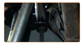
Tighten the fastener connecting the stabilizer link to the stabilizer bar. Use a combination spanner #18. Use a drive socket #18. Use XZN #6. Use a torque wrench. Tighten it to 55 Nm torque.
