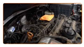
Detach the crankcase ventilation hose from the oil filler neck.
