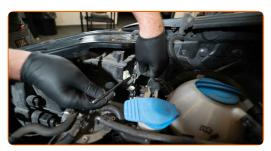
Detach the bulb holder by turning it by ~30°. Remove the holder from the headlight mounting seat.
