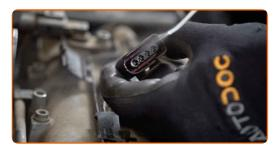
Treat the ignition coil tip. Use high-temperature grease. Use a flat screwdriver.
