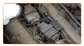
Pry up the ignition coil. Use a crowbar. Use a flat screwdriver. 10
