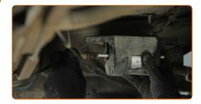
10 Install the new fuel filter together with its bracket.
