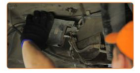
Remove the fuel filter. Use a flat screwdriver.
