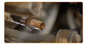
Screw on a new tie rod end. Use a vernier caliper.
