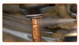
Connect the tie rod end to the steering knuckle.
