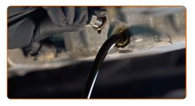
Replacement: engine oil and filter – VW Passat B5 Estate (3B5). Tip from AUTODOC:
