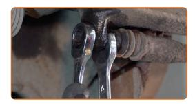
Remove the brake caliper. Use a crowbar.
