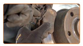
11 Remove the brake disc.
