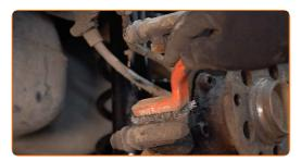
Replacement: brake discs – VW Passat B5 Estate (3B5). Tip from AUTODOC:
