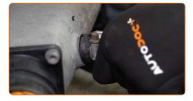
Fasten the clamp on the crankcase ventilation hose. Use a drive socket #7. Use a ratchet wrench.
