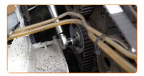
Clean the engine valve cover mounting seat. Use all-purpose cleaning spray.
