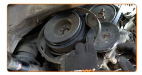
Clean the alternator fasteners. Use a wire brush. Use WD-40 spray.
