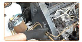
Tighten the fasteners of the upper timing cover. Use a drive socket #13. Use a torque wrench. Observe the recommended tightening torque.
