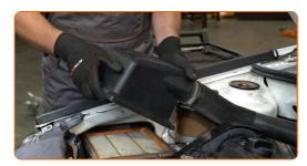
Unscrew the fasteners of the air distribution housing assembly. Use a drive socket #7. Use a ratchet wrench.
