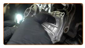
Tighten the water pump fasteners. Use a drive socket #10. Use a torque wrench. Observe the recommended tightening torque.
