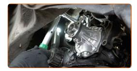
Treat the mounting seat of the vacuum pump pulley. Use all-purpose cleaning spray.
