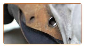
Detach the crankcase ventilation hose clamp. Use a drive socket #7. Use a ratchet wrench.
