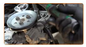
Clean the mounting seat of the timing belt tensioner pulley. Use a wire brush. Use all-purpose cleaning spray.
