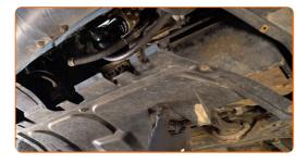
Put a waste oil container with at least 5 l capacity under the drainage hole.
