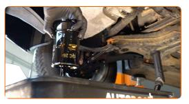
Replacement: engine oil and filter – VW Passat B3/B4 Box Body / Estate (315, 3A5). Tip from AUTODOC experts:
