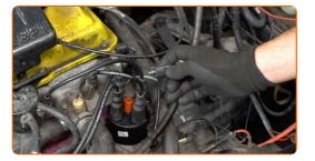
Replacement: ignition leads – VW Passat B2 Variant (33B). Tip:
