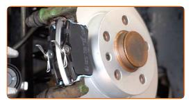
Replacement: brake pads – VW Passat B2 Variant (33B). AUTODOC recommends:
