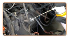
Connect the spark plug wires to the distributor cap.
