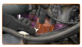
Disconnect the spark plug wires from the distributor cap.
