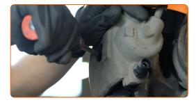
11 Remove the brake caliper.
