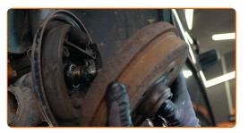
Replacement: wheel bearing - VW Passat B1 Hatchback (32). Tip:
