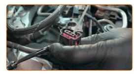
Attach the engine wiring harness connectors.
