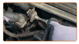
6 Unscrew the brake fluid reservoir cap.
