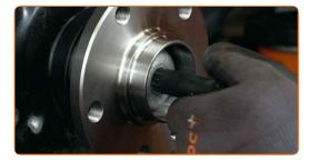
Install the hub bearing protection cap. Use a hammer.
