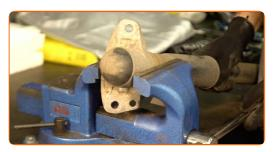
Remove the protective cap of the shock absorber mount. Use a crowbar.
