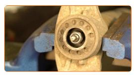
Clean the shock absorber rod fastener. Use a wire brush. Use WD-40 spray.
