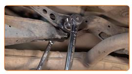
Clean the exhaust system fastener. Use WD-40 spray.
