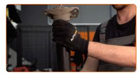
Screw the shock strut piston rod upper fastening. Use a shock absorber socket DDNº6. Use a drive socket #17. Use a torque wrench. Tighten it to 25 Nm torque.
