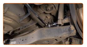
Unscrew the upper fastener of the shock absorber. Use a drive socket #16. Use a tap wrench.
