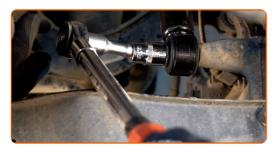
Remove the support from under the arm.
