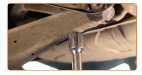
Clean the exhaust system fastener. Use WD-40 spray.
