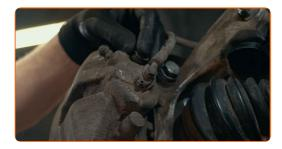
Install the brake caliper retaining spring. Use a crowbar.
