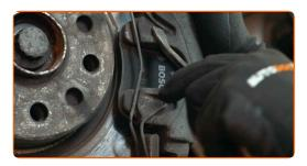
Remove the brake caliper.
