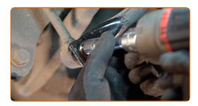
Unscrew the fastener connecting the stabilizer link to the control arm. Use a drive socket #15. Use a ratchet wrench.
