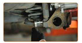
Secure the rear axle beam. Use a hydraulic transmission jack.
