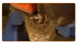
Remove the shock absorber piston rod fastening. Use a drive socket #17. Use a ratchet wrench.
