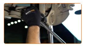
9 Remove the fastening bolt.
