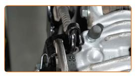
Undo the brake bleeder screw. Use a combination spanner #10.
