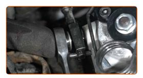
Tighten the fastener connecting the brake pipe to the brake caliper. Use a drive socket #13. Use a torque wrench. Tighten it to 40 Nm torque.
