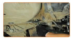
Remove the support from under the arm.
