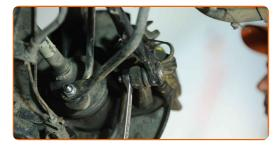
Clean the fasteners connecting the control arm to the subframe. Use a wire brush. Use WD-40 spray.
