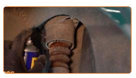
Unscrew the upper fastener of the shock absorber. Use a drive socket #13. Use a ratchet wrench.
