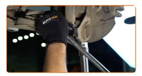
9 Remove the fastening bolt.
