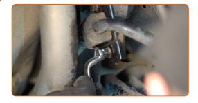
Unscrew the fasteners connecting the stabiliser link to the stabiliser bar. Use a combination spanner #15. Use a drive socket #15. Use a ratchet wrench.
