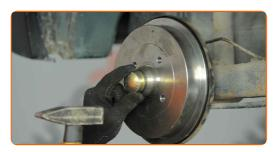
Clean the wheel rim mounting seat. Use a wire brush. Treat the surface where the wheel rim contacts the brake drum. Use copper grease.
