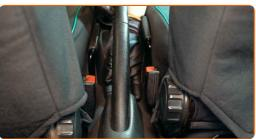
Loosen the parking brake cable. Use a combination spanner #10.
