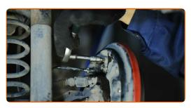
Remove the brake cylinder from the backplate. Use a flat screwdriver.
