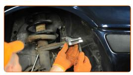
Loosen the lock nut securing the tie rod end to the tie rod. Use a combination spanner #14. Use a combination spanner #22.
