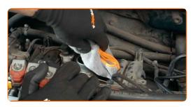
Install the air filter housing and fasten it. Use a Phillips screwdriver.
