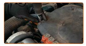
Remove the air filter housing.
