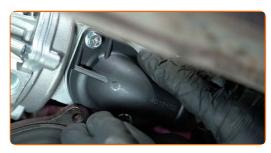
Tighten the thermostat housing fasteners. Use a drive socket #10. Use a torque wrench. Tighten it to 13 nm torque.
