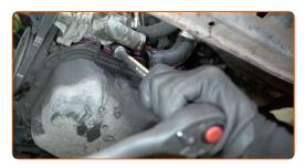
Remove the thermostat housing.
