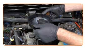
Pour coolant in the coolant reservoir.
