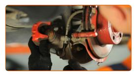
14 Remove the brake pads.
