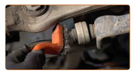
Unscrew the fastener connecting the stabilizer link to the stabilizer bar. Use a combination spanner #16.
