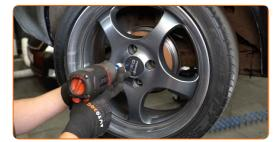
Lower the car and working in a cross order, tighten the wheel bolts. Use wheel impact socket #17. Use a torque wrench. Tighten it to 110 Nm torque.
