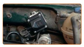
Tighten the ignition coil fastening. Use a drive socket #10. Use a torque wrench. Tighten it to 7 nm torque.
