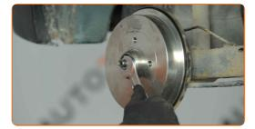
Install the cotter pin of the hub bearing fastening nut. Use a hammer. Use nippers.
