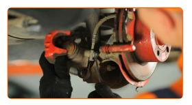
14 Remove the brake pads.
