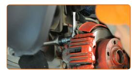
Remove the brake caliper. Use a flat screwdriver.
