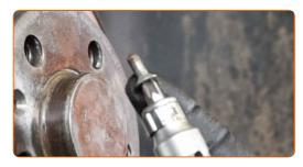
Remove the brake disc.
