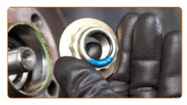
Remove the hub and the bearing together, since they are made as an assembly. Use 3-Arm Gear Puller.
