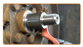
Clean the ABS sensor. Use a nylon cleaning brush. Use all-purpose cleaning spray.
