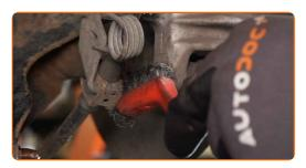
9 Unscrew the brake caliper fasteners. Use a combination spanner #13. Use a combination spanner #15.
