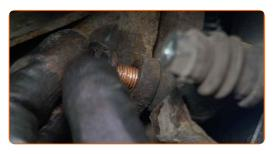
Tighten the brake caliper bracket fasteners. Use HEX No.H8. Use a torque wrench. Tighten it to 65 Nm torque.
