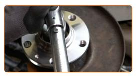
Install the hub bearing cap. Use a rubber mallet.
