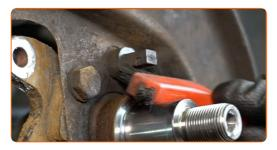
Install the new wheel hub together with the bearing. Use a bush and bearing driver set. Use a hammer.
