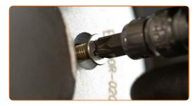
Tighten the brake disc fasteners. Use a Phillips screwdriver. Use a torque wrench. Tighten it to 4 Nm torque.
