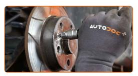
19 Remove the fastening bolt.
