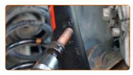
Remove the brake caliper bracket.
