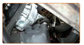
Replacement: engine thermostat – VW New Beetle Hatchback (9C1, 1C1). Tip:
